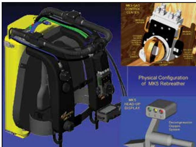
Figure 12. The Cis-Lunar Mk5P rebreather used during the Wakulla 2 project.
