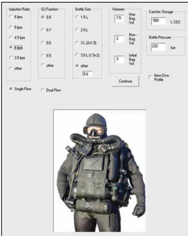
Figure 16. Semiclosed-UBA definition screen. John R. Clarke figure.
