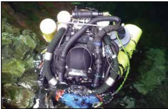
Figure 2. Cave diver Sandy Varin, in the entrance to the Pearse resurgence in NZ, wears a twin rebreather system built by combining a backmounted rEVO unit with a Classic Inspiration scrubber and circuit attached to the diver's left side. Photo by Richard Harris.
