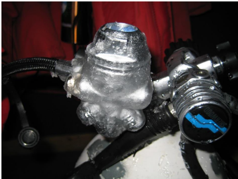
Figure 11-2 Normal salt water ice accumulation encrusting a regulator 1st stage.
