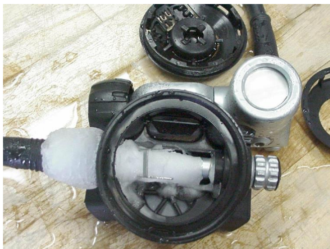
Figure 11-1 Ice accumulation in a 2 nd stage regulator after free flow.
