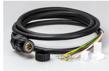
Cable is delivered with terminals Molex 08-55-102 crimped, connectors Molex 22-01-3037 are packed separately, to be mounted after passing through cable gland.
