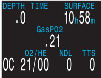
Here is an example of a simple OC air dive. It will help to introduce the screen displays as the diver progresses, the dive starts, the depth increases. The display is showing the computer programmed for open circuit (OC) air.
