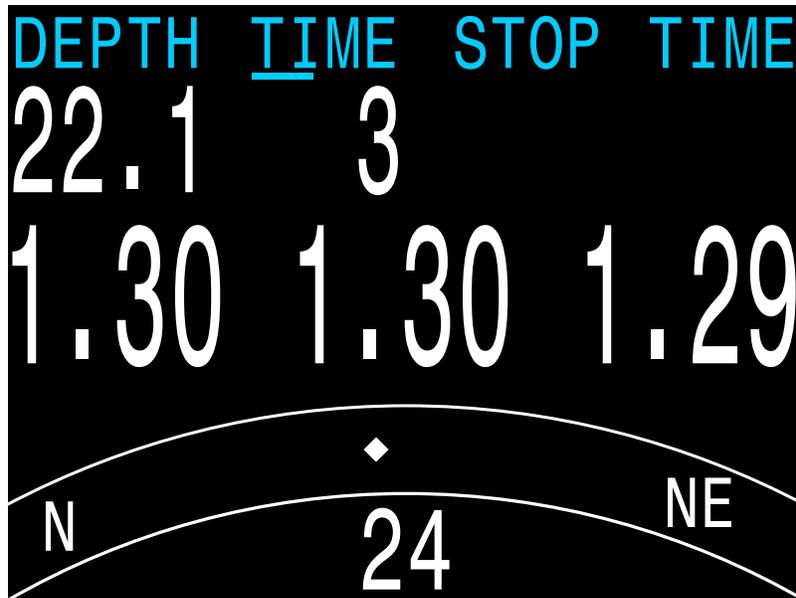
The NERD 2 contains a tilt-compensated digital compass in the eyepiece. The compass indicates the direction you are looking.
