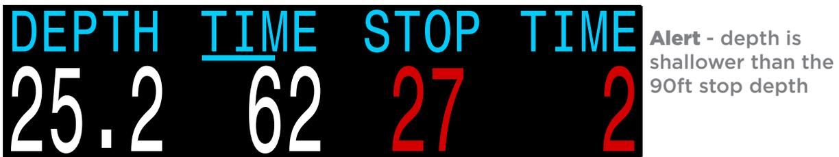
By default the NERD 2 uses a 3m (10ft) last stop depth. At this setting, you may perform the last stop at 6m (20ft) with no penalty. The only difference is that the predicted time-to-surface will be shorter than the actual TTS since off-gassing is occurring slower than expected.
