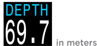
Note: If the depth shows a Flashing Red zero or shows at depth at the surface, then the depth sensor needs service.
