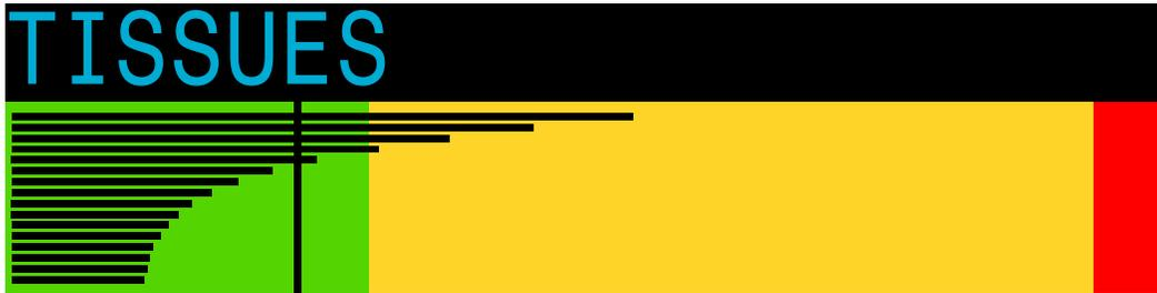
The tissues bar graph shows the tissue compartment inert gas tissue tensions based on the Bühlmann ZHL-16C model. Note that VPM-B also tracks tensions in the same way.
