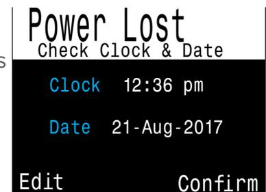
The NERD 2 uses a highly accurate quartz crystal for time keeping. Expected drift is about 1 minute per month. If you notice drift, it is easily corrected in the **System Setup Menu**.
