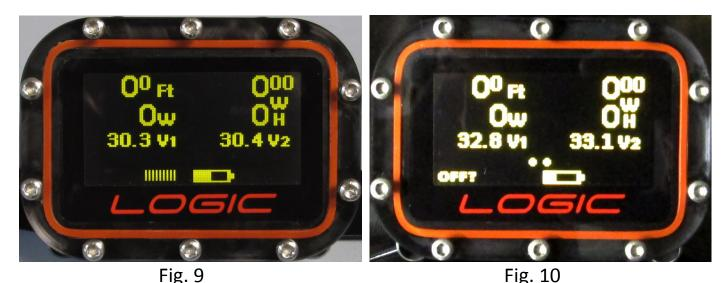
**Depth** (top left corner): Displays the depth in feet or meters with 0.1 unit precision. The depth is compensated for altitude, provided the display is turned on before entering the water. If the display is turned on while under water, it will revert to standard sea level calibration. The depth is accurate to 425ft (130m) and accuracy may decrease slightly when below that. The Sentry housing is rated for 660ft (200m),
