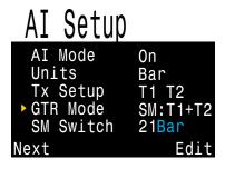
GTR and SAC are only based on one tank, or on two tanks in sidemount configuration. Note that for sidemount the tanks must be of identical volume for SAC to be accurate.
