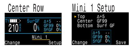
The Perdix 2 has a mini display function that allows it to show 3 pieces of information in each of the left and right custom slots at the expense of font size.
