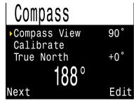
**60°**, **90°**, **or 120°**: Sets the range of the compass dial that is visible on the main screen. The actual amount of arc that there is room for on the screen is 60°, so this may feel the most natural. The 90° or 120° settings allow a wider range to be seen at once. The default is 90°.
