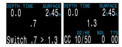
For closed circuit diving the Perdix 2 operates in internal PPO2 mode. This mode is used to calculate decompression for an unconnected rebreather.
